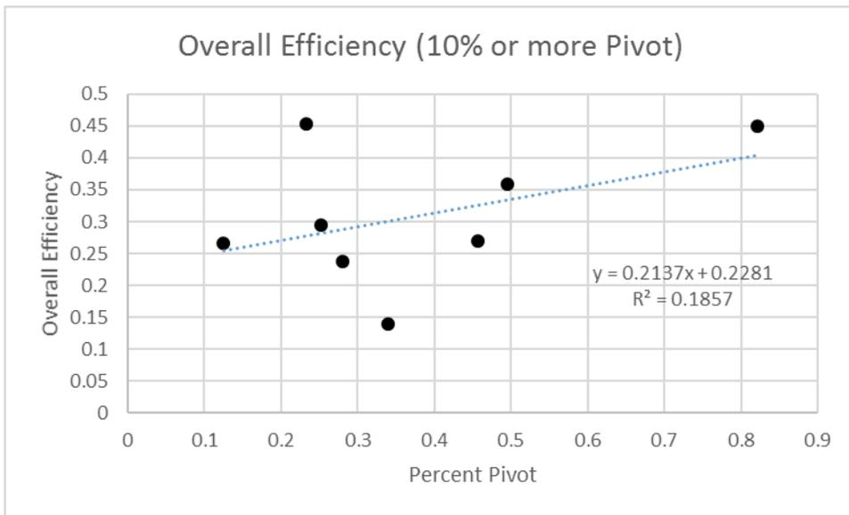
Figure 8: Average Overall Efficiency per Diversion Site vs Percent Pivot (10% or more Pivot)
