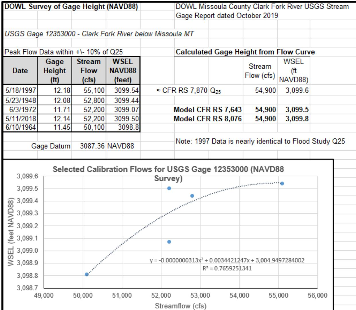
**Figure 8. 1D Hydraulic Model Calibration to Clark Fork River Stream Gage 12353000**
