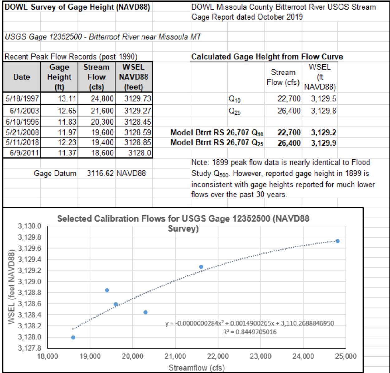
**Figure 9. 1D Hydraulic Model Calibration to Bitterroot River Stream Gage 12352500**
