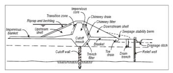
Figure 5: Potential Seepage and Internal Erosion Mitigation Features
