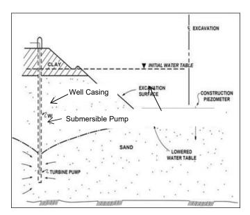
Figure 7 - A Deep Well Installation (Adapted from [5])
