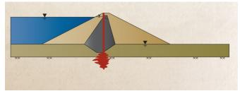
Figure 10: Foundation Grouting from the Dam Crest
