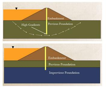
Figure 7: Potential Cutoff Wall Configuration
