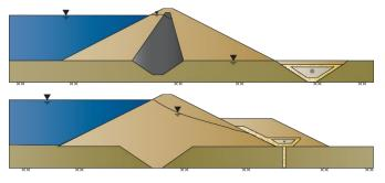
**Figure 8: Potential Foundation Filter Configurations**
