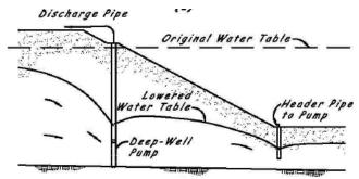
Figure 8 - Supplemental Dewatering Required If Low Permeability Boundary Exists Near Bottom of Excavation [4]
