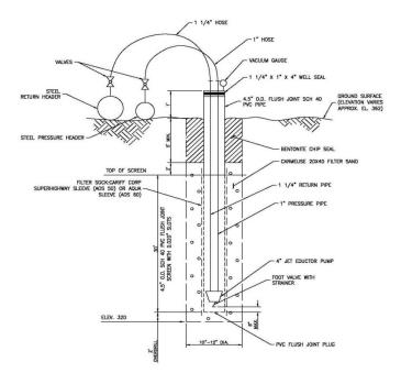
Figure 6 - Typical Design Detail for an Eductor Well (AECOM Technical Services)
