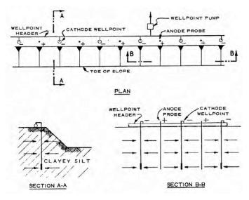
Figure 12 - An Electro-Osmosis Installation [5]
