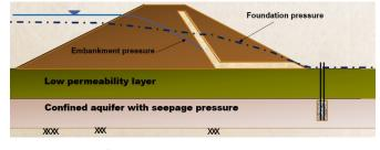
Figure 11: Relief Well Schematic
