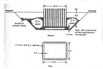
Figure 3: Example of More Complex Sump Installation [3]
