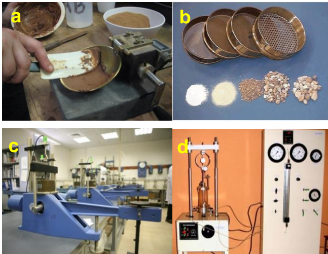
Assortment of soil testing equipment: (a) Atterberg Limits, (b) Sieve Analysis. (c) Consolidation. (d) Triaxial Shear
