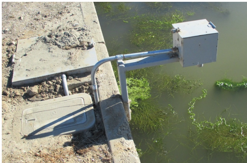
Figure 12. Ultrasonic sensor measuring the water level upstream of a weir in West Stanislaus Irrigation District alongside a submersible pressure transducer (not shown)
